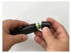
Screw the negative cap onto the Echo Cell Cartridge.
