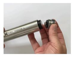
Install the end cap on the Echo transmitter.
