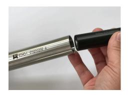
Install the Echo Cell Cartridge into the Echo transmitter positive side down.
