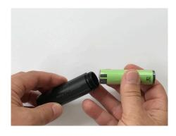
Place one lithium battery into the Echo Cell Cartridge positive side down.
